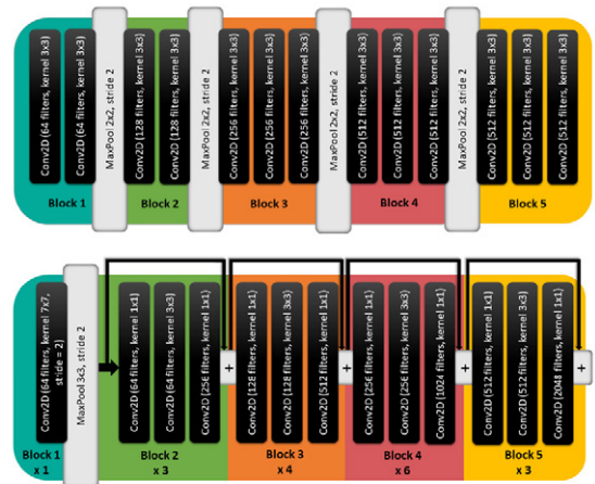
Fig. 6. Details regarding each used pretrained model for the face recognition stage : (Top) VGG16, (Bottom) RESNET 50.
