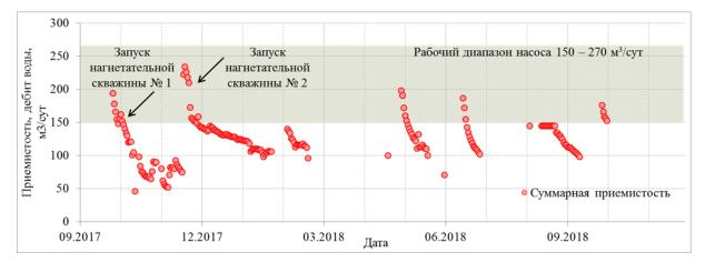
Injectivity, water flow rate, m³/day Start of injection well №1 Start of injection well №2 Pump operating range 150-270 m³/day Total injectivity Date
