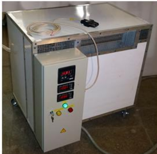
Figure 3 - Combined electrical device with heat accumulation
