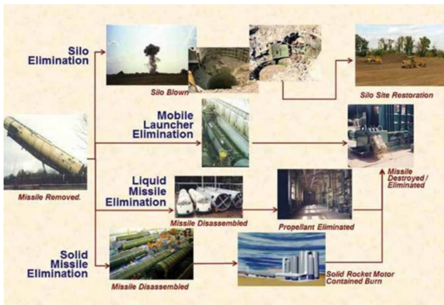
Figura 4. Proceso de Desmantelamiento de un ICBM. Fuente: Harahan, J. (2014). With Courage and Persistence - Eliminating and Securing Weapons of Mass Destruction with the Nunn-Lugar Cooperative Threat Reduction Program . Defense Threat Reduction Agency, p. 160.
