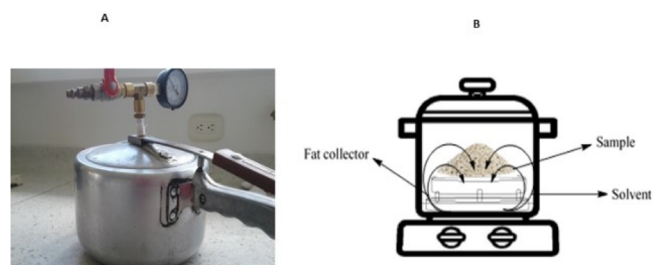
Figure 1. a) Conventional pressure vessel, b) internal pressure vessel system
