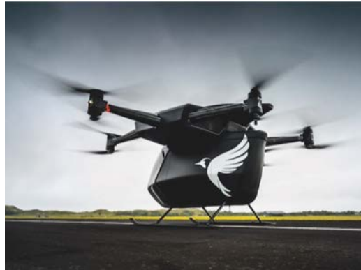
Figure 33: The Vertical Aerospace's latest prototype, Seraph, can fly at speeds of up to 80km/h and carry 250kg, the equivalent of three passengers
