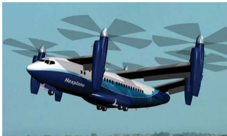
Figure 40: Hexplane, a Six-Engine Airliner-Helicopter Hybrid
