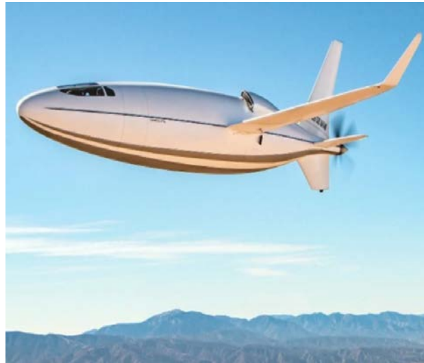
Figure 22: The laminar-flow design of the Celera 500L gives it a 4,500-mile range while its operating costs are about a sixth of competitive business jets
