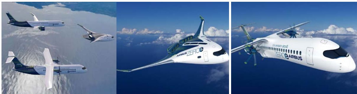
Figure 21: The project includes a hydrogen turboprop, which is rotated by a modified gas turbine engine
