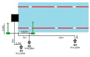
Figure 2. Location of cameras (C1, C2 and C3) and reference systems
