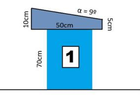
Figure 1. Starting platform or block used during the measurements
