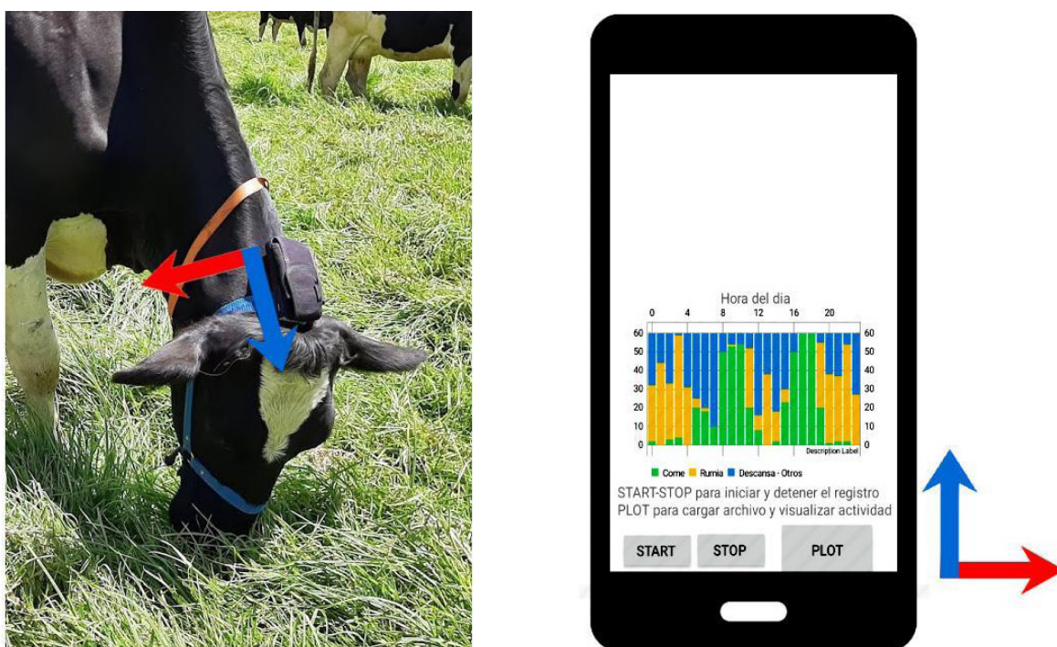
Figure 2. Cow wearing the device and the app screen. Arrows show the correct position of the smartphone on the cow's head.
