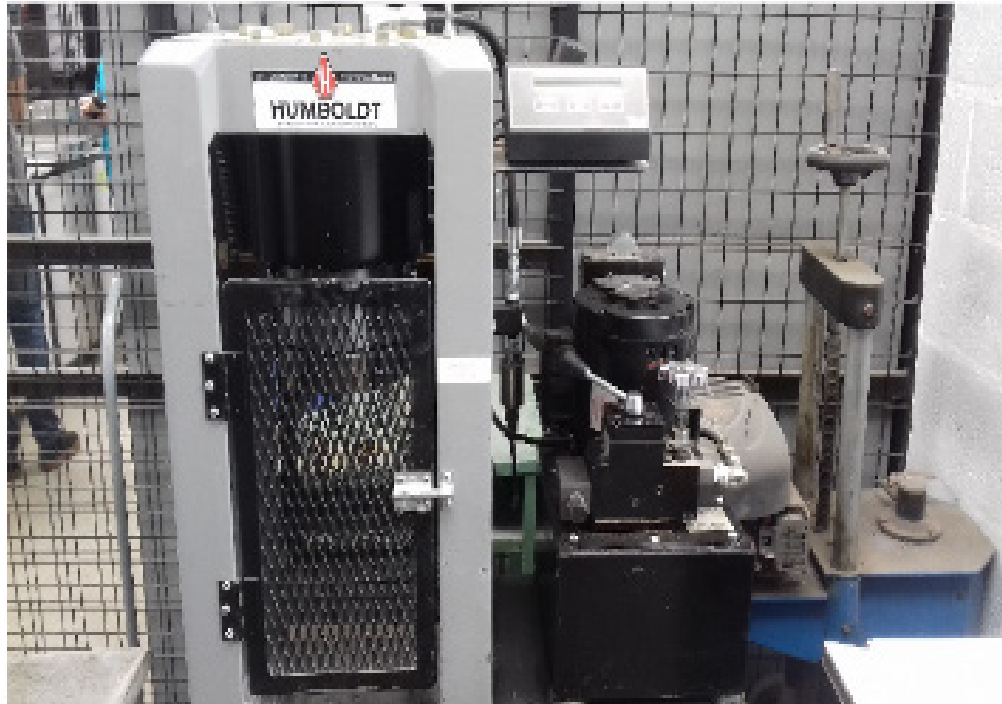
Fig. 2. Humboldt compression machine
