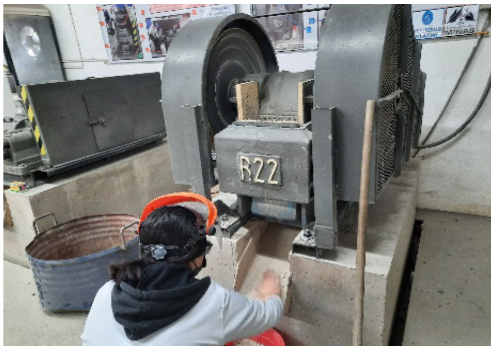
Fig. 3. Crushing the specimens in the R22 jaw crusher
