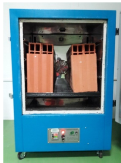
Figure 3. Dried process of the samples in the oven Gabrielli. Source: The authors.
