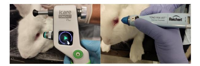
**Figure 3.** Rebound (TONOVET Plus<sup>®</sup>) and applanation (TONO-PEN VET<sup>®</sup>) tonometers. The image on the left shows the TONOVET Plus<sup>®</sup> tonometer and the image on the right shows the TONO-PEN VET<sup>®</sup> tonometer, both of them about to perform measurement intraocular pressure in New Zealand rabbits.
