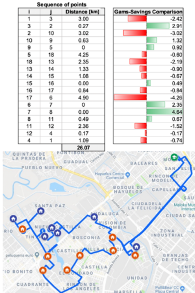
Figure 6. Route map for the Kennedy area and its comparison with the TSP model (in Gams).
