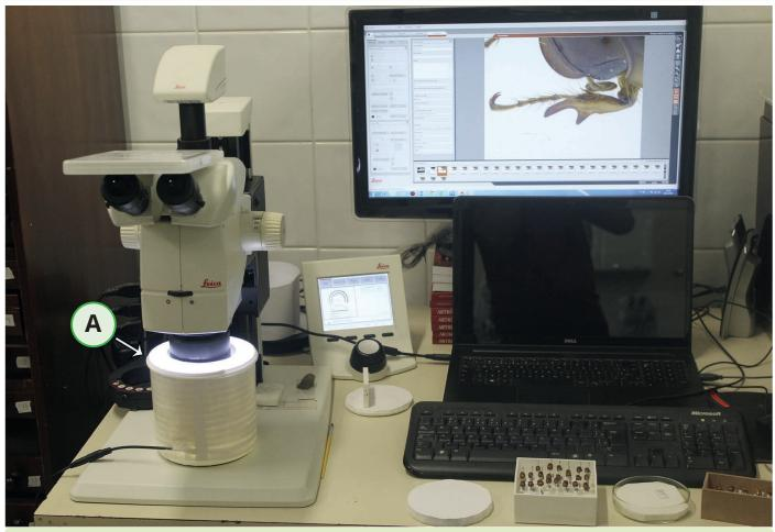
Figure 3. Stereomicroscope self-assembly, model Leica M205 C: A) circular LED dome lighting system.
