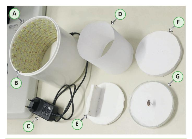
Figure 1. Circular LED dome lighting system: A) circular illuminator; B) ribbon of white lamps of LED; C) power source; D) white paper filter; E) support to fix the insects in lateral view; F-G) supports to fix the insects in dorsal view.
