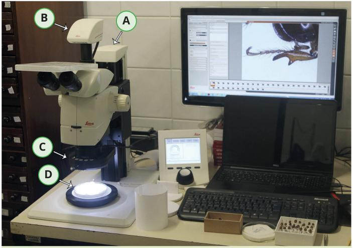
Figure 2. Stereomicroscope self-assembly, model Leica M205 C: A) stereomicroscope; B) digital camera; C) fully integrated ring light; E) support with pinned insect.
