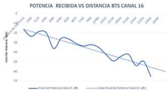
Figure 3. Relation received power versus distances for Calatrava on channel 16. Source: own.
