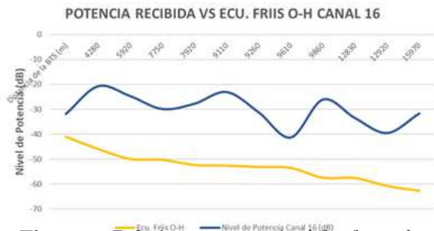
Figure 9. Relation power waited for from the model of Okumura-Hata for Green Cross Canal 16. Source: own.
