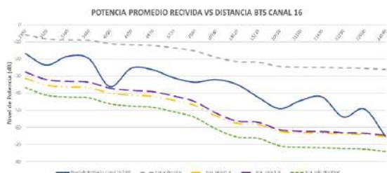
Figure 14. Compilation models Okumura-Hata, Stanford, Xia-Bertoni versus data measured for Calatrava Canal 16. Source: own.
