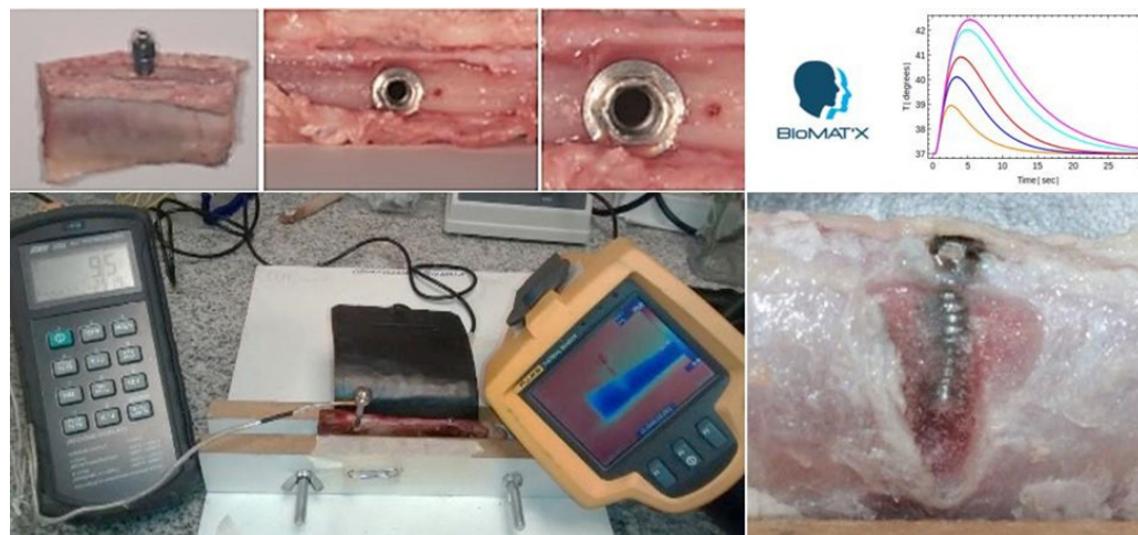
Figure 2. BioMAT'X ex-vivo X'PLANT 3Ss model – thermal change monitoring/recording (imaging and quantification, in real-time) performed using a CorDEX TP3R ToughPix DigiTherm Digital Thermal Camera.
