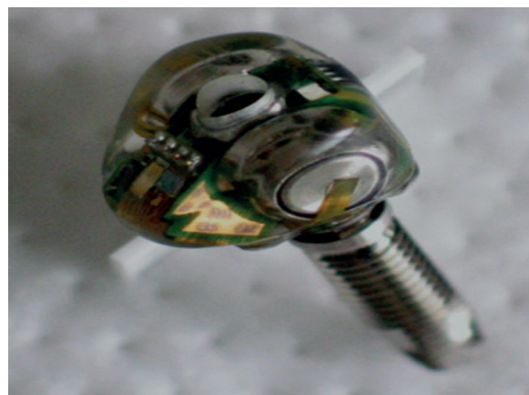
Figure 4. Active dental implant: Artificial tooth containing wetness sensor, battery and an electrostimulation unit for stimulating secretion of saliva
