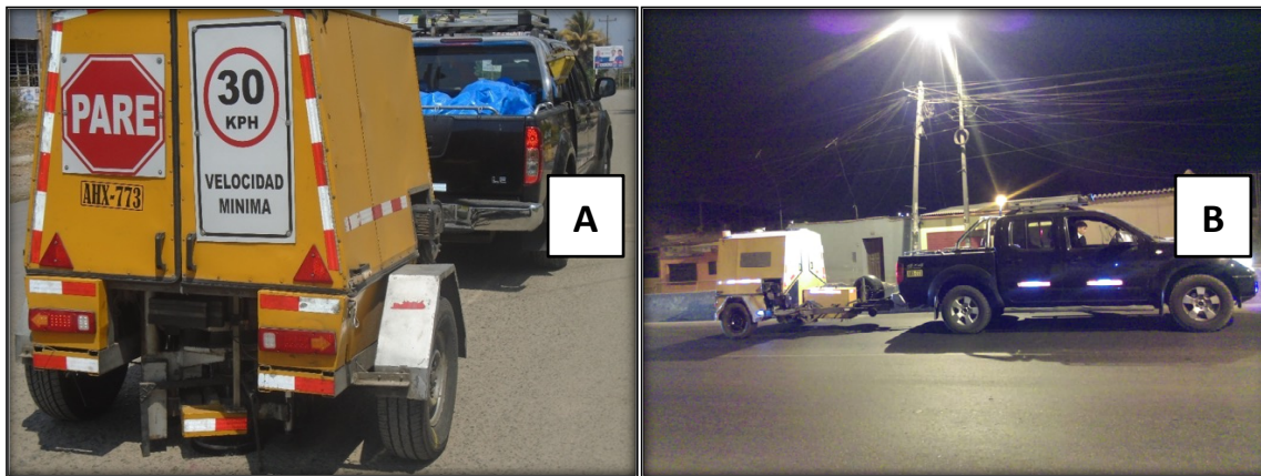
Figure 2. Impact deflectometer KUAB - 150 coupled to a trailer transported by a pickup truck, this device is dynamically loaded and meets ASTM D 4694-96 requirements.
