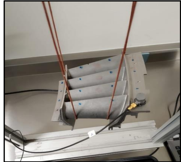
Figure 1. Set of blades used to get the vibrational modal model.
