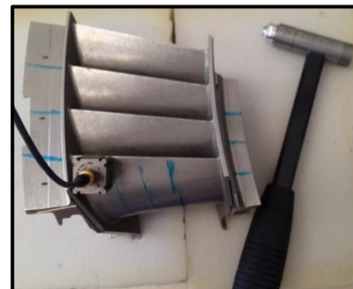
Figure 3. Experimental setup for the impact test.
