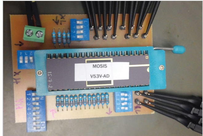
Figure 13b. Integrated circuit of 8 bits Wallace tree FP multiplier. Testing PCB.
