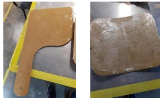
Fig. 20. Armrest and seat manufactured.
