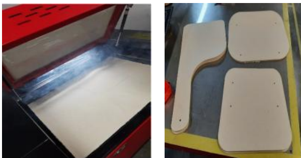
Fig. 18. Laser cutting of parts.
