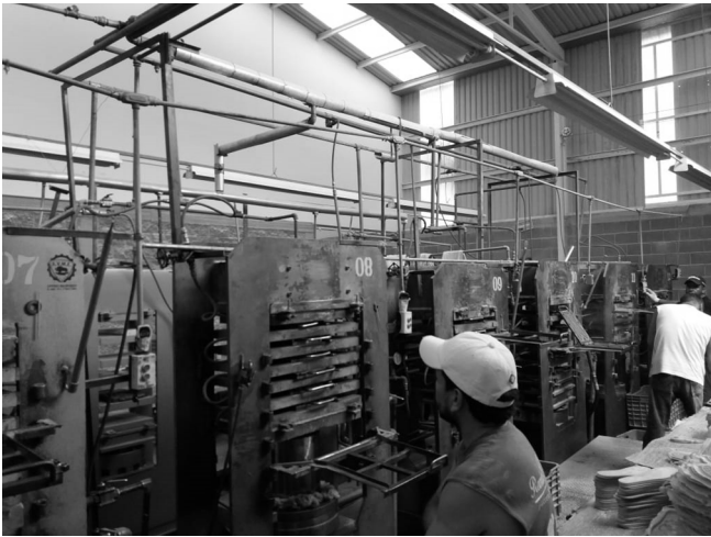
Figure 3. Vulcanization process in the press area Source: The authors
