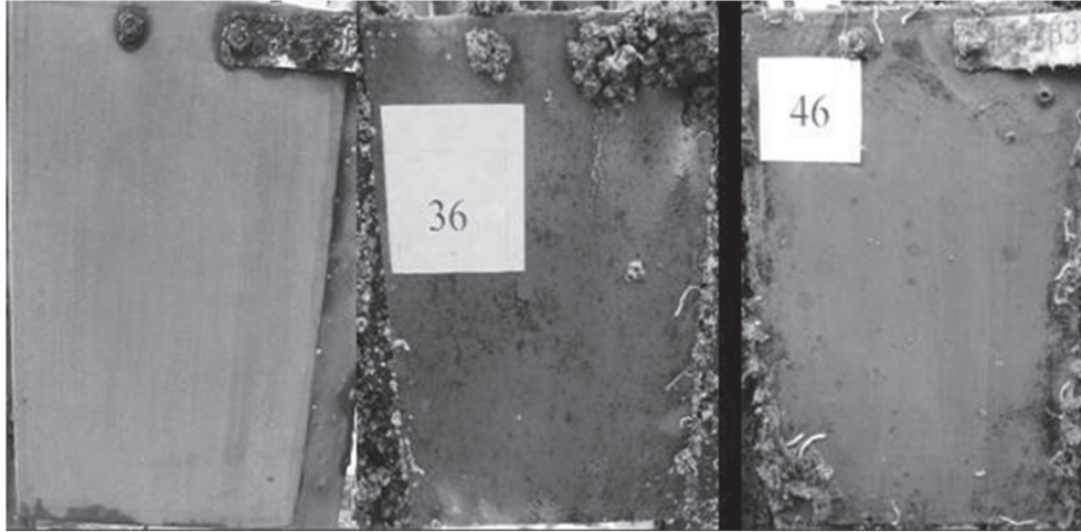
Figure 3. Metallic panels painted with formulation 17 after 51, 240, and 471 days (depth: 2.60 m)
