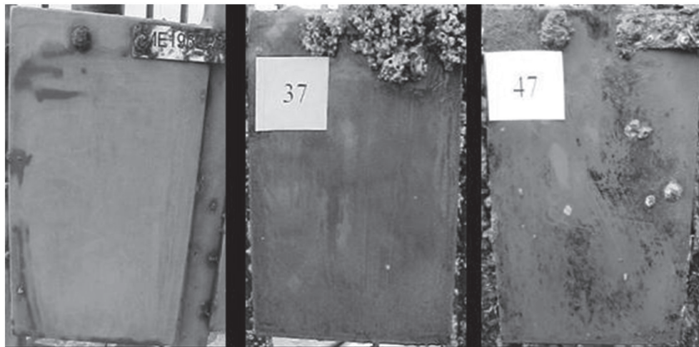
Figure 4. Metallic panels painted with formulation 19 after 51, 240, and 471 days (depth: 2.60 m)
