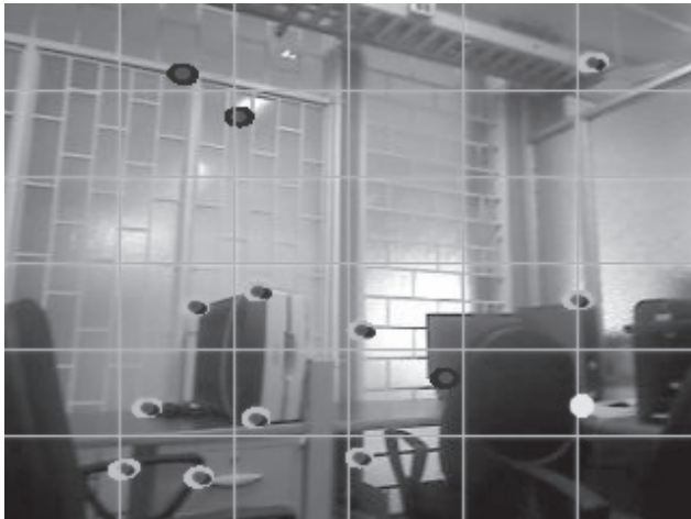
Figure 3. Prediction of the feature location in the image plane (red points). The ellipses represent the prediction uncertainty.
