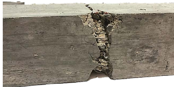
Figure 8. Fragments confined in a beam specimen due to the anchoring provided by knotted PET profiles placed in a bidirectional fiber matrix. Source: The authors
