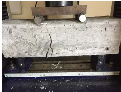
Figure 4. Concrete Flexural Resistance using a simple concrete beam with load in the middle third of the clearing. NMX-C-191-ONNCCE [15]. Source: The authors
