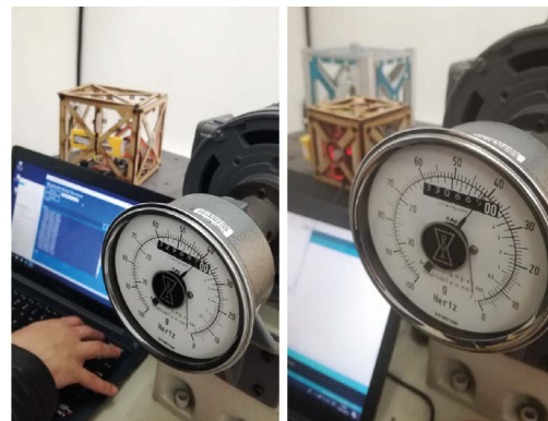
Figure 24. Non-standard wood and aluminium CubeSats coupled at Vibration test bench.
