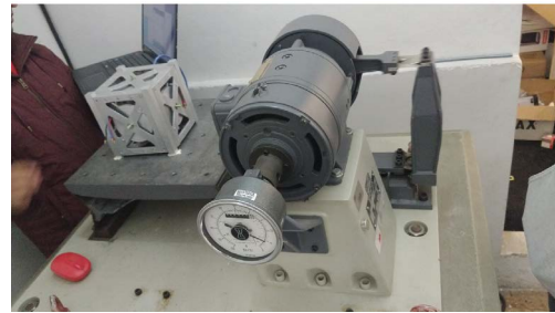
Figure 23. Non-standard CubeSat coupled at Vibration test bench. Source: Cortés-García et al. (2019).
