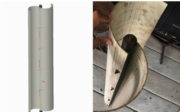
Figure 1. AutoCAD vs Hardware of Blades and Shaft.
