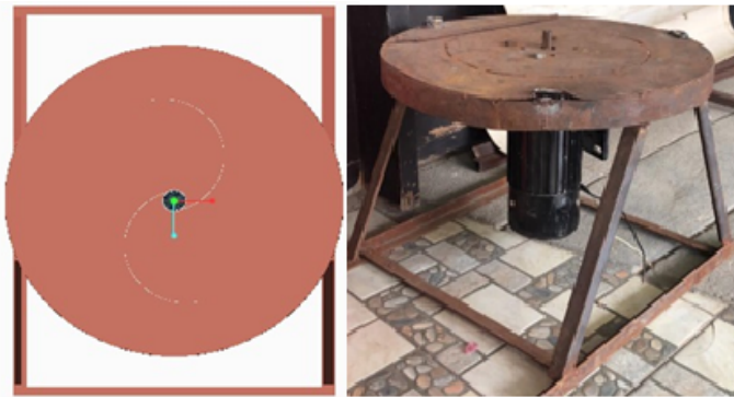
Figure 2. AutoCAD vs Hardware of Base of Turbine.
