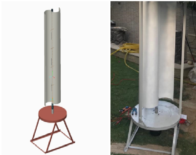
Figure 6. AutoCAD vs Hardware of S-rotor.
