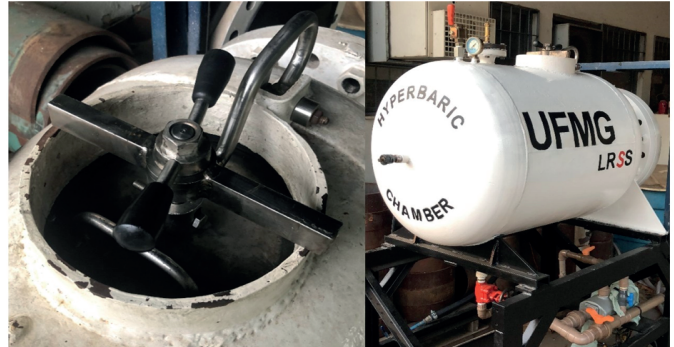
Figure 13. Modifications of the LRSS hyperbaric chamber (left), overview of the LRSS hyperbaric chamber (right)
