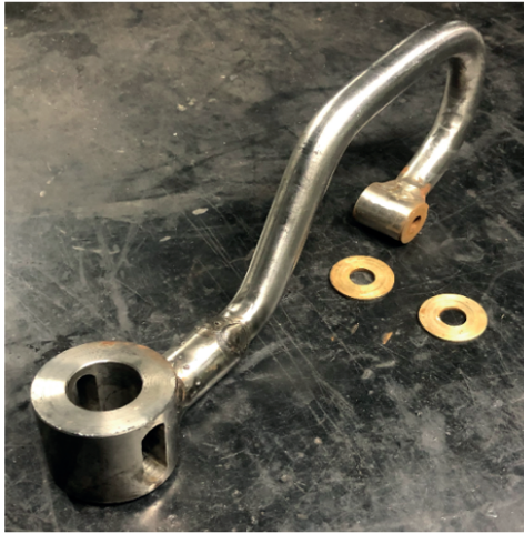
Figure 11. Articulated arm and manufactured washers
