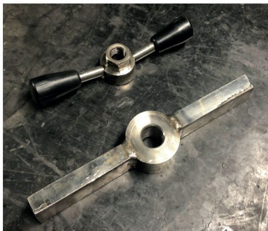
Figure 12. Rod and handwheel with welded nut
