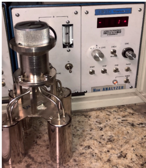
Figure 2. Chromatography and capsule used in the hydrogen diffusible test in the LRSS
