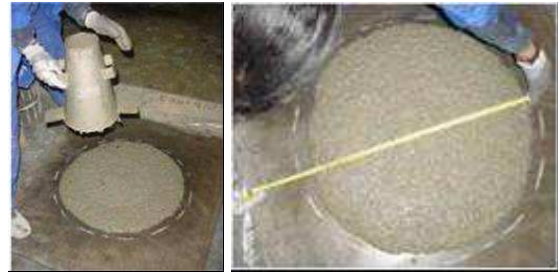
Figura 5. Ensayo de Escurrimiento [1] Figure 5. Slump flow test [1]
