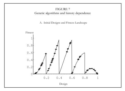
A typical algorithm consists of three parts. (i) Selection: each string is selected with a probability proportional to its fitness value. (ii) Crossover: in a pair of selected designs (strings), a position along the string is chosen, and the right and left part of each string are swapped. And (iii) mutation: each gene (a particular digit in the string) is changed at random with a small probability.
