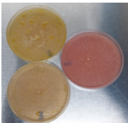
Figure 2. Phenol red method: pink plate corresponds to glucose assay and yellow plates corresponds to flaxseed oil assay. Source: The Authors.
