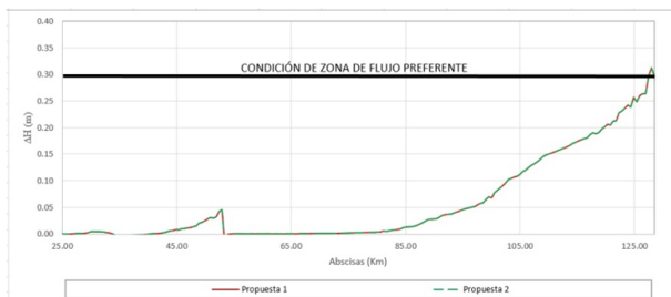
Figure 7. Variation of the water level for a Rt of 100 years between the proposals Riparian Buffer Zone and the hydrological component. Section: Timba River – South Interceptor Channel.
