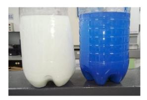
Figure 5. Samples after 1 hour of Electrocoagulation
