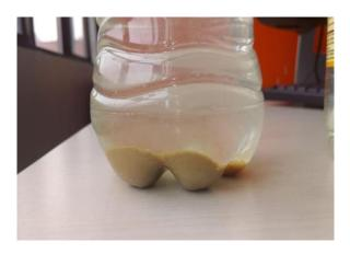
Figure 8. Roller washing water after one hour of treatment in the electrocoagulation equipment and one night of decantation
