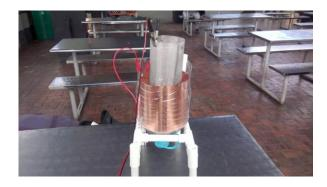
Figure 2. Scale prototype for electrocoagulation water treatment
