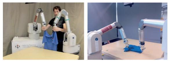
FIGURE 2. Experimental scenario of the task of teaching a bimanual robot to fold garments, in this case a polo shirt, by means of an initial demonstration (left) followed by autonomous learning for reinforcement (right).
