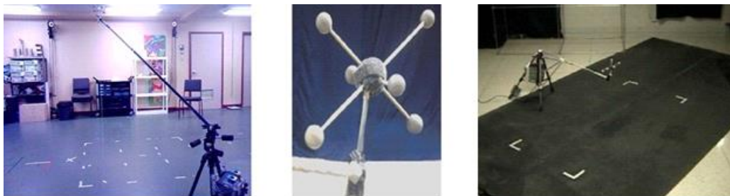
Figure 3 Device for metrological characterization and configuration of the cluster of markers used.
