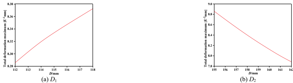
Figure 9. Response diagram of design variable to maximum valve body deformation. Source: The Authors.
