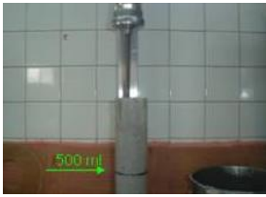
Fig. 2. Marsh Cone and Time in the Marsh Cone [7]
