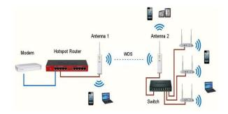
**Figure 3.** Hotspot router Mikrotik together with antennas connected WDS.
