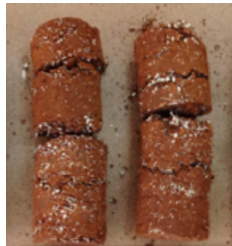
Figure 9. A picture of two tested CL with 20% CNC-W specimens.
