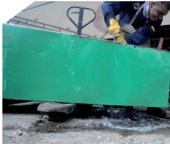
Fig. 9. Application of antifouling paint.
