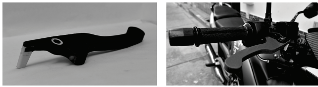
Figure 13. Phase 3: demolding, final form and assembly. Source: The Authors.
