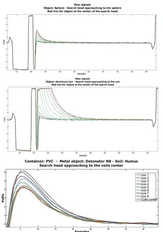
Figure 6. Metal Detector Prototype. Objects: Sphere, Aluminum Can, and Home-made landmine with detonator (Up to down). Las señales están dentro de medio período (periodo: 1 kHz, and 71 [sg/sample) Source: The Authors.
