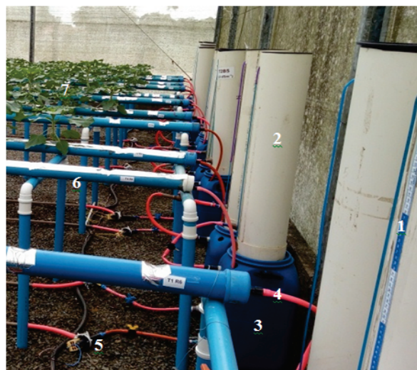
1 – Ruler, 2 - Reservoir to measure water consumption, 3 - Nutrient solution tank, 4 - Tube for return of excess solution, 5 - Electric pump, 6 - Hydroponic profile, 7 - Sunflower seedlings.
