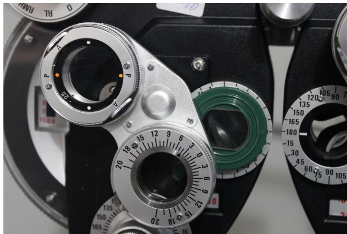
Figure 1. Example of a base-out prism of unknown power attached to the phoropter using Velcro
