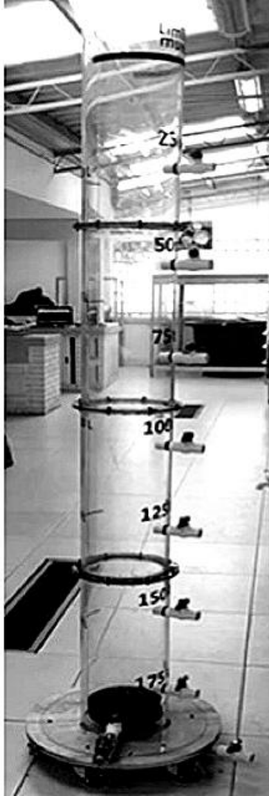
Figure 1. Sedimentation tower built for this research. Source: The Authors.
