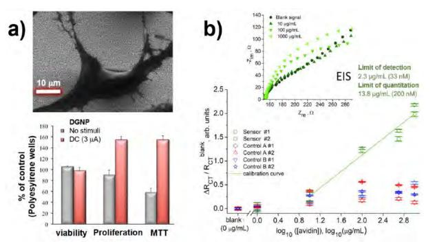
**Figure 4.** Biomedical applications of DGNP films. a) Top: SEM micrograph of a murine MC3T3-E1 preosteoblast (mouse boneforming cell) adhered to DGNP substrates. Bottom: MC3T3-E1 cell viability, proliferation and metabolic activity calculated via MTT (3-(4,5-dimethylthiazol-2-yl)-2,5-diphenyltetrazolium bromide) test, expressed as function of percentage of control (standard cell culture plates). The cells were cultured on DGNP substrates with and without application of DC periodic stimuli.
