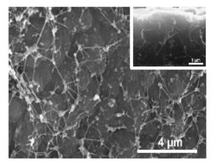
**Figure 2.** The hybrid surface after diamond overgrowth. CNTs can still be seen protruding from the diamond surface and embedding into it. The inset corresponds to a cross section view of the same structure where CNTs, surrounded by a continuous NCD layer, are evident.
