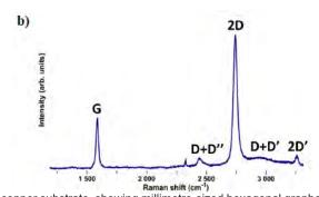
Figure 6. a) SEM image and b) Raman spectrum of CVD graphene on a copper substrate, showing millimetre-sized hexagonal graphene domains and a spectrum typical of single-layer graphene.
