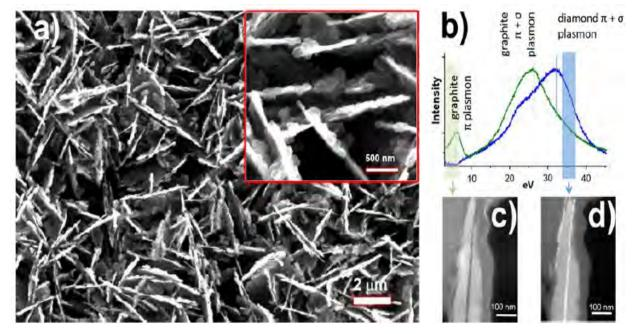
**Figure 3.** a) SEM micrographs of DGNP thin films. b) Low energy region of the electron energy loss spectra acquired from a nanographite (green) and nanodiamond (blue) sites. Energy windows are adequately chosen to form the energy-filtered images of c) and d), where the brighter contrast identifies nanographite and nanodiamond, respectively.
