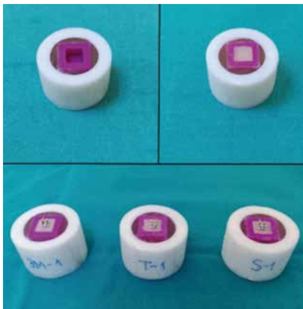
Figure 1. The cylindrical specimens, A: Empty mould embedded in acrylic rod. B: Mould filled with composite. C: Specimens with bonded brackets from different groups.
