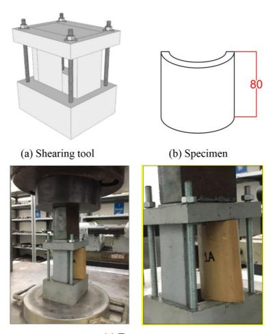
(c) Test set-up
