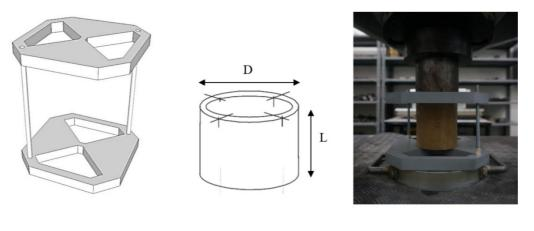
(a) Shearing tool (b) Specimen (c) Set-up
