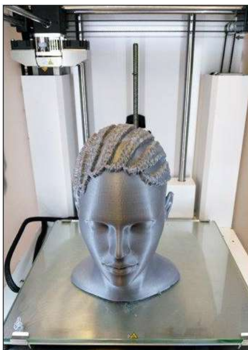
FIGURE 11 – 3D printer rendering a virtual cornrow design as a mannequin head Source: by permission of the author
