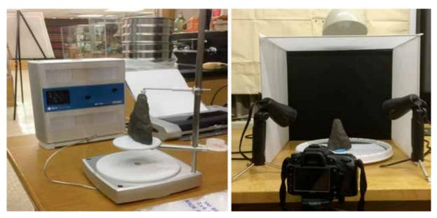
Figure 11: Left, NextEngine 3-D scanner; right, photogrammetric workstation.
