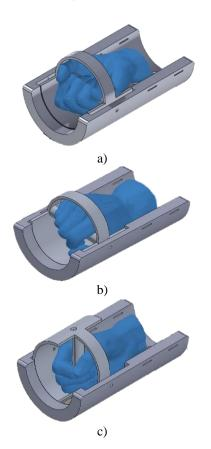
Figure 7. Pronosupination positions: a) Supination, b) Pronation, c) Intermediate.
